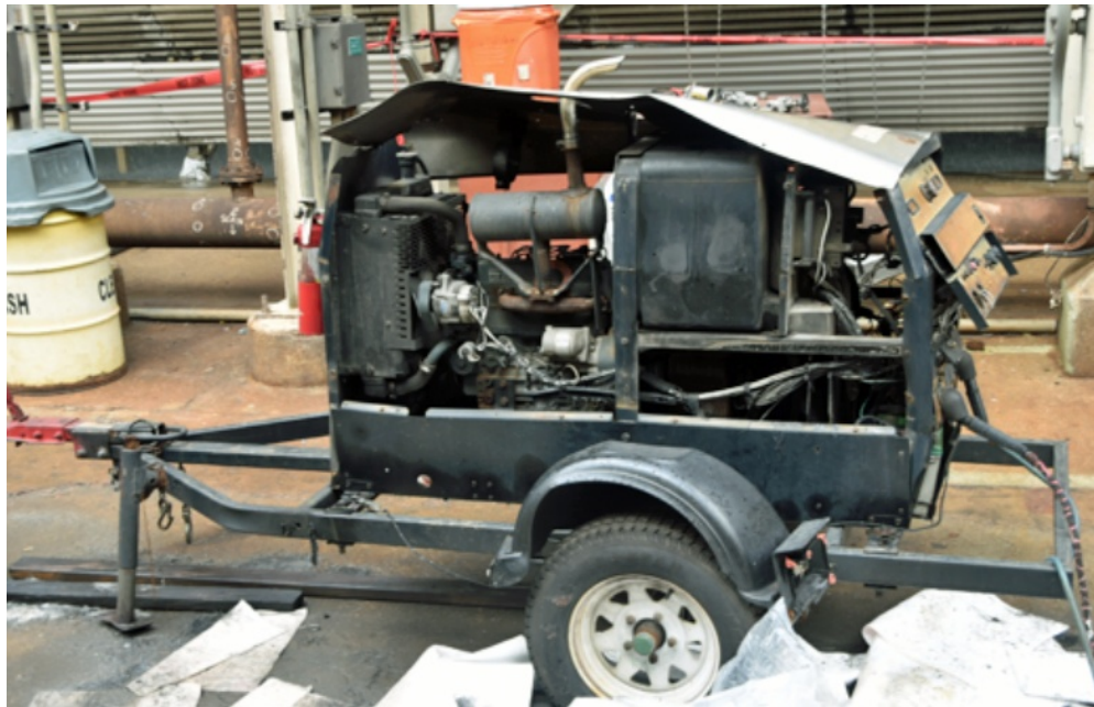
Figure 4. Welding machine that was the likely ignition source of the isobutane vapor cloud.
